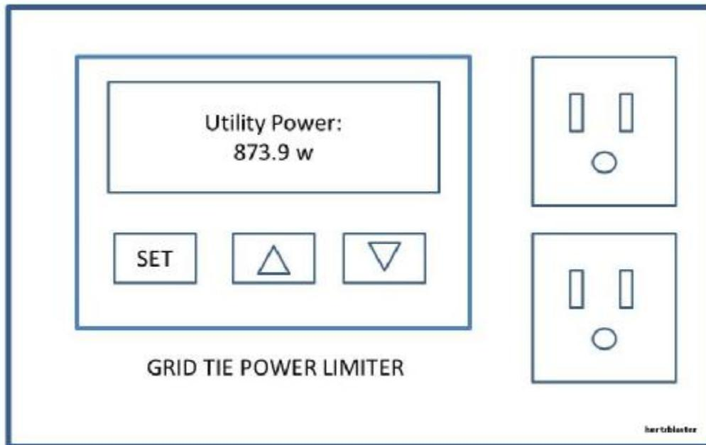
To reset the Utility Total, just press the up button for a few seconds and you will be prompted yes or no to reset. Press up or down button to select either yes or no, and then press SET to reset .
