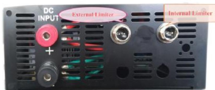
Attention:For external limiter mode.Need to long press the SET button when initial power on the GTIL system after all connections are done.Due to grid failure or malfunction,GTIL system will able to auto restart after grid recover.
