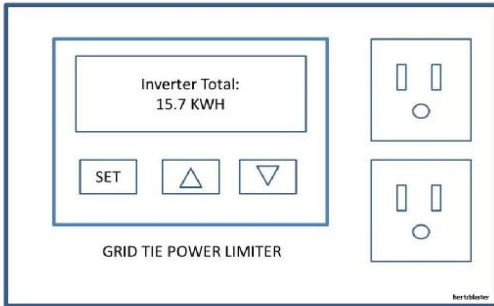
4.3.9. Connect the GTIL power output to the LM AC receptacle using the supplied cable. Turn on the disconnect switch/dc breaker of solar panel.
