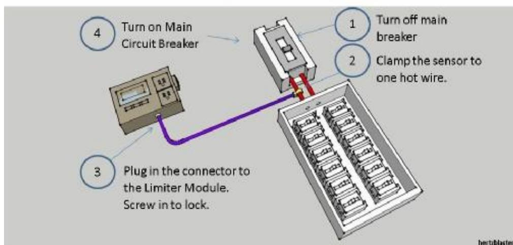
4.3.2 Connect the LM module to grid. Using the terminal block, use at least wire no.12 AWG (20A ampacity - wire not included in the package) and connect to 20A circuit
