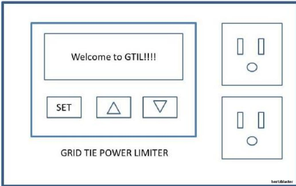
4.3.8. After initialization, LCD will display Utility Power, which is the actual power or total load in real time. Press the up and down buttons to display the Inverter Power, Utility power, Utility Total KWH and Inverter Total KWH. Inverter Power should read zero initially.
