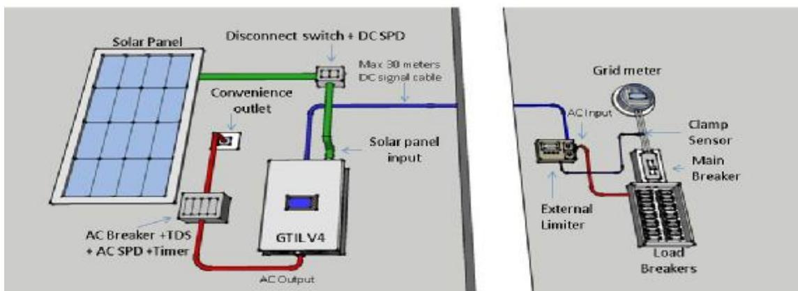
4.1. The installations of the GTIL system are shown above, The ac plug can either connect to the nearby AC socket or plug into the limiter socket, the dc signal cable can reach max 30 meters length so that you can able to install the inverter far away from the limiter module. The ideal installation is that the limiter install near the GTIL. The GTIL unit and the Limiter Module are placed close to each other. The signal wires will be short, as supplied with the unit.
